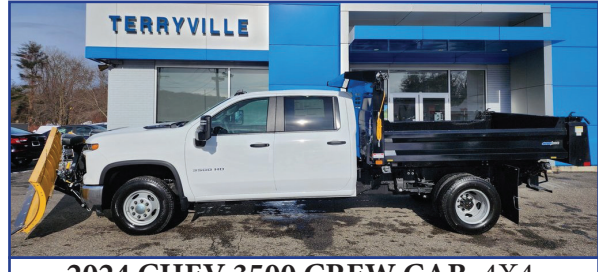
2024 CHEV 3500 CREW CAB. 4X4, Duramax Diesel, Automatic, 2-3 Yard Dump Body, #30312
