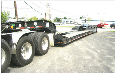
2005 FONTAINE TL50 LOWBED TRAILER. 25' Level Deck, 18" Deck Height, 3 Axle, Air Ride, Alum Wheels, Recently Reconditioned, Very Good Condition. Call For More Information.
