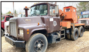
1970 MACK DM-400. Turbocharged Scania Diesel, 10 Speed, 8,000 Lb. PTO Driven Crane, Runs Excellent. $9,500
