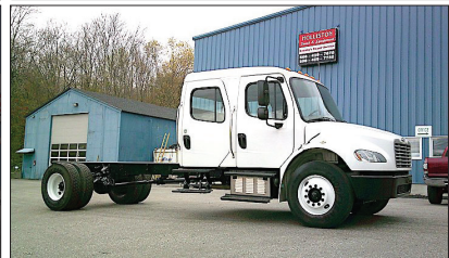
2016 FREIGHTLINER M2: CUMMINS ISB-250HP, 63K MILES, EXHAUST BRAKE, ALLISON 3500RDS AUTO, 26K GVW, SPRING SUSP., SINGLE FRAME, 11R 22.5 TIRES, AIR-BRAKES / SEAT, A/C, PTO CAPABLE, 126" CAB TO AXLE, 174" OF FRAME, 236" WB. $50,000
