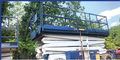
SKY JACK SJ 92-50 SCISSOR LIFT. Kubota Diesel, Runs Great, New Tires, Extendable Platform, 4 Outriggers
