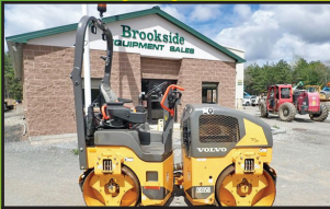
2021 VOLVO DD35B: 786 Hours, 54" Smooth Double Drum, Vibratory, 3 Cyl Kubota Turbo, 48 HP, 8.2k Lbs, Stk#CO507, $38,500
