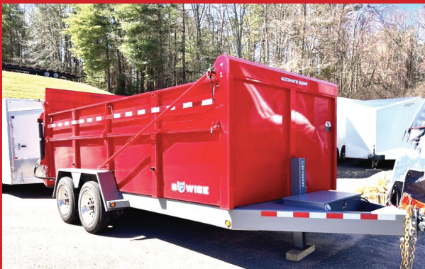
B WISE ULTIMATE DU17 DUMP TRAILER. 82" x 16', Heavy Duty Hoist w/ 5" Cylinder, #T14096, Sale Price $25,997
