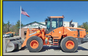
2017 DOOSAN DL220-5: 3,326 Hours, 3 Yard, Cab W/ A/C, Hydraulic Coupler W/ 3rd Valve, 6 Cyl Doosan Turbo, 28k Lbs, Stk#LO165, $94,500
