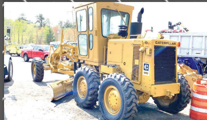
1989 CAT 120G MOTOR GRADER. EROPS, 13' Moldboard, Articulating Center, 13R24 Tires, $36,500.
