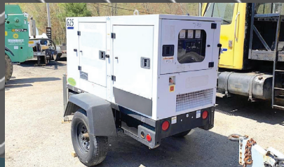
2018 DOOSAN GX25. 25kw Generator, Doosan Diesel Engine, 15k Hours, One Owner, Pintle Hitch, Electric Brakes, 3 Phase, Work Ready, $9,500.
