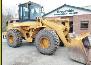
1994 CATERPILLAR 938F: 9,582 Hours, 3.4 Yard, Cab W/ Heat, Aux Hyd, 6 Cyl Cat 3116 Turbo, 140 HP, Very Good Rubber, 30K Lbs. stk#LO192, $32,500
