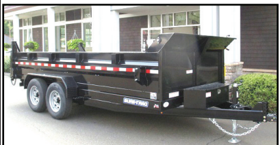
SURE-TRAC 7 TON LOW PROFILE DUMP TRAILER. 6'10" x 16', Combination Barn Door Spreader Gate, Side Steps, #362181
