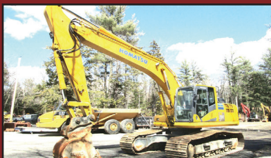
2013 KOMATSU PC290 LC-10. 7360 Hrs, Long Stick, JRB Cplr, Aux. Hyd., Recent Track Chains & Sprockets, 42" Bucket, $95,000.
