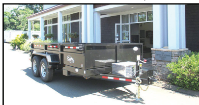
CAM SUPERLINE 13.2K HD LOW PROFILE DUMP TRAILER. 6' 9" X 14', Tubular Main Frame, #526610
