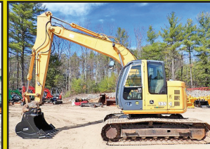
2008 JOHN DEERE 135C RTS: 6,339 Hours, 39" Bucket, Hydraulic Coupler, 1-Way Aux. Hydraulics, A/C, Reduced Tail Swing, 4 Cyl Isuzu Turbo, 90 HP, 31K Lbs, stk#XC890, $52,500
