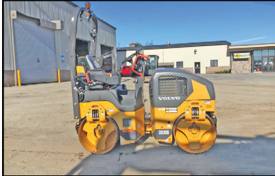
VR181 2018 VOLVO DD30B. 49 HP, Only 20 Hours, 49" Double Drum, Pressurized Water System, OROPS, $45,300.
