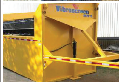
VIBROSCREEN SCM-75 HEAVY DUTY SCREENER Vibrating Head w/2 Decks , Up to 300 Cubic Yards/ Hour, 50 HP Diesel Engine, Ideal For 6 Yard Loader, Fifth Wheel Hitch, Single Axle, Double Wheels, Hydraulic Landing Gear, Gross Weight 22,000 LBS Tongue Weight 8,540 LBS Rental Rates: Daily $700 • Weekly $2,100 • Monthly $6,000
