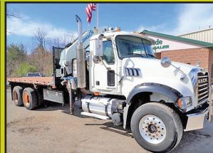
2007 MACK GRANITE CTP713: 123,332 Miles, 10 Whl Knuckle Boom Crane Truck, Gormach 28200-E6, 20 Ft Flatbed Dump, Mack MP7-370, Mack 10 Spd, 18K F, 44K R, Stk#TK651, $59,500
