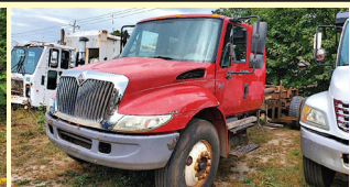
2003 IH 4400 CREW-CAB HOOK-LIFT, 109K MILES, DT466, ALLISON 3500 RDS, 40K GVW, GAL BREATH 30K HOOK WITH 54/62 HOOK - HEIGHT DOES 16' BOXES, CALL FOR MORE INFO!
