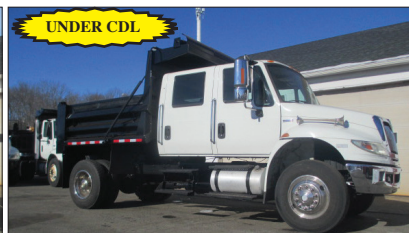
2008 INTERNATIONAL 4300: DT530/MAX 9-275HP, 31K ORIG. MILES, EXHAUST BRAKE, ALLISON 3500 RDS AUTO, 26K GVW, SPRING SUSP., 5.64 GEARED RATIO, LOCK DIFF., 10R 22.5 TIRES, SINGLE FRAME, A/C, PTO, 9" STEEL DUMP, 3 CHUTES, AIR-GATE, ELECTRIC TARP, PINTLE. $49,000
