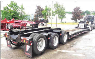
2008 FONTAINE 55 TON, FLD, Currently Being Reconditioned, 25' Deck, 18" Deck Height, 2 Pin Position, Air Ride, Tri Axle, 275 Rubber, Strobes, Call For More Information.
