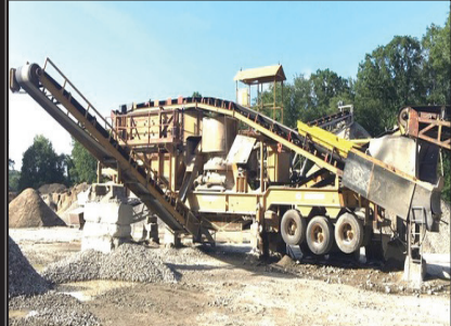
1988 ALLIS CHALMERS 45 HYDRO. 45 Inch Cone, New Manganese & Hydro Set Seals, 200 HP Electric Motor, 5X16 Triple Deck Screen, Closed Circuit Conveyors, Triple Axle Chassis, Serial #C-53463, $130,000 . Gales Ferry, CT. Chris, 860-460-0767 or Chm@TerraFirmaus.com
