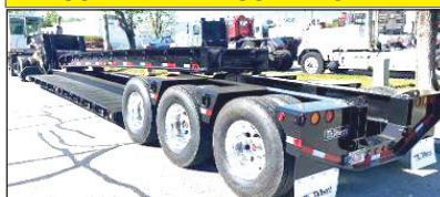
2009 TALBERT 70 TON DROP SIDE RAIL, Severe Duty, 26' Steel Deck, 9' Wide, With 26' Beam Insert, 30,000 Lb Axles, 3 Axle, Set Up For 4th, Spring Ride, 315 Rubber, One Owner, Completely Reconditioned, Sandblasted And Painted. New Seals, Brakes, Bearings, Hubcaps And Decals. Call For More Information.
