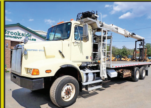
2006 WESTERN STAR 490SA: 172,152 Miles, 10 Wheel Sheetrock Boom Truck, IMT 16000S3 Boom, 42 Ft, 5285 Lb Cap, 24'6" Flatbed, AWD, Cat C13, 410 HP, 21.5K F, 46K R, T-Ride, 15,864 Engine Hrs, Stk#TK147, $39,900
