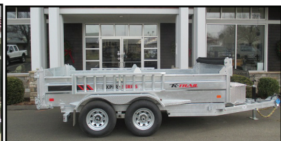
K-TRAIL DUMP TRAILER. 6' x 12', Ramps, Combo Doors, LED Lights, 9875 lb GVW, #JM019175
