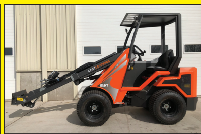
CAST 23T. 23HP Kubota Diesel, Extendable Boom, Aux Hydraulics
