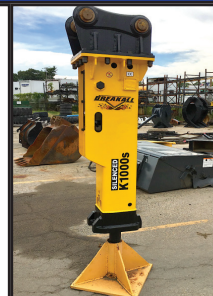
NEW BREAKALL K1000 HYDRAULIC HAMMER, Operating Weight 1,168 lbs., Impact Rate BPM 480-850, Impact Energy 1,500 lbs., Carrier Weight 15,000-27,000 lbs., Fits A 307-311 Excavator. $11,950 or $249/Month. 401-785-9800
