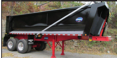
2020 RHODES. 26' Steel Dump Trailer AR450, Dual Hinge High Lift-Gate, 70,000# Single Point, Electric Cover. Call 401-434-5900
