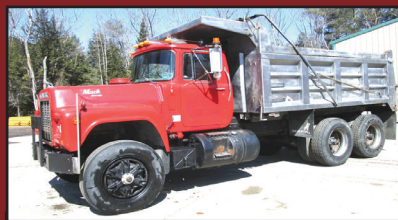
1986 MACK RD686. 300 Motor W/Brake, 2 Stick 6 Spd, 18R+44R Camelback, New Dble Frame & Frog Leg, 14' Body, Pintle & Air, $24,000.
