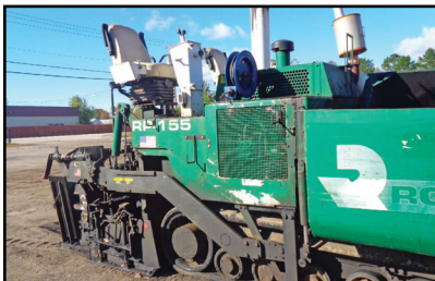
8764 2006 ROADTEC RP155 8 FOOT CARLSON SCREED. 14" Augur, Hystat, 155 HP Deere Diesel, Rubber Tracks At 40%, $25,500
