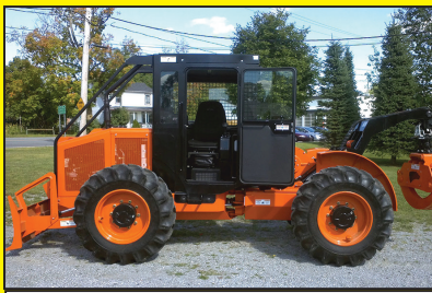
AWASSOS MD80. Log Skidder, 84HP, 12,000 lbs, Hydostatic Drive, Grapple, Winch, 7.5'-8.5' Wide
