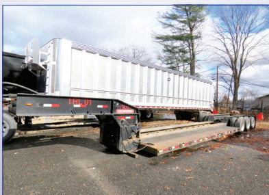
1989 ROGERS 60 TON LOW BED TRI AXLE DROP SIDE TRAILER: 22.5 Tires @70%, 70% Brakes, NEW Suspension. 24' Deck. Sand Blasted & Painted.
