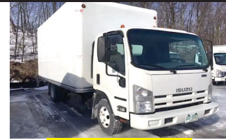
2014 ISUZU NPR HD: 4HK1-TC, 215HP., Diesel, Automatic, Lease Maintained, Alum. Lift-Gate, 16' All Fiberglass Unicell Body, E-Tracks, Leaf Spring Susp., 150WB, 16" HD Radials, Only 56,850 Miles And Much More ! $39,500 #7E7002252
