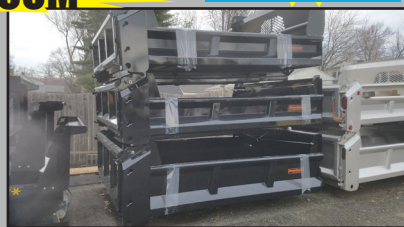
DOWNEASTER STEEL DUMP BODIES IN STOCK 2-3 YARD & 3-4 YARD, PAINTED BLACK, DOUBLE-ACTING HOIST, LED LIGHT PACKAGE
