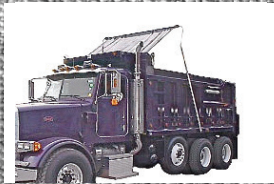
FLIP TARP / SPRING SYSTEMS Can Be Mounted On Truck Bodies Up To 48 Feet In Length And Are Available In Manual Or Fully Automatic Systems. Variety Of Motor, Tarp, And Mounting Options. Optional 18 Oz. Tarp Or Hot Top Material Available. Call With Your Specs.
