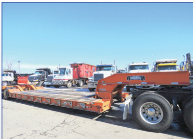
1996 ROGERS 35 TON Low Bed. Non Ground Bearing, Air Ride, 22.5 Tires, 22' x 102" Deck. Very Good Condition. $18,500
