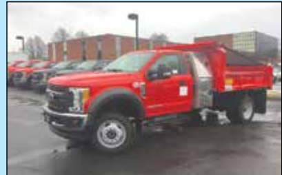
2017 FORD F550. Diesel, 4x4, 9' Crysteel Dump Body, 1 Pack, Power Group, #HDA06380
