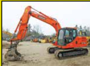
2013 Doosan DX140 LCR-3: 1,510 hours, 36" bucket, hydraulic thumb, hydraulic coupler, very good u/c, a/c, 6 cyl Doosan turbo, 32k lb size class, stk#XC094, $79,900
