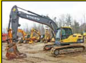
2013 Volvo EC220DL: 3,764 hours, 42" bucket, aux hyd, hydraulic coupler, good u/c, a/c, 6 cyl Volvo turbo, 51k lb size class, stk#XC299, $87,500
