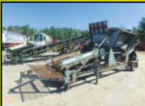
2003 Rawson 3618: 2,510 hours, towable conveyor screen, grizzly, 102" by 42" hopper, 16" belt, 2 cyl Honda gas, 20 hp, comes w/ 30 ft radial stacker, stk#SC402, $26,500
