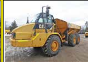
2011 Caterpillar 730: 11,776 hours, 30 ton, 6x6, artic., a/c, 6 cyl Cat C11 Acert turbo, 23.5R25 good rubber, stk#HT069, $129,500
