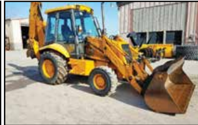
8655 1996 JCB 214. COUPLER, 3RD VALVE, GP BUCKET ON FRONT, EXTENDA-HOE, 30" DIG BUCKET ON REAR, 4X4, FULL CAB, W/ HEAT. MACHINE RUNS GREAT! $18,500
