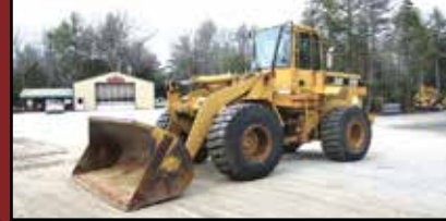
1994 CAT 936F. 11,200 Hrs, ACS Hyd. Coupler, 3rd Valve, 3.5 Yd. Bucket, Matched 20.5 X 25 Radials @ 80%, Runs Very Good, $30,000.
