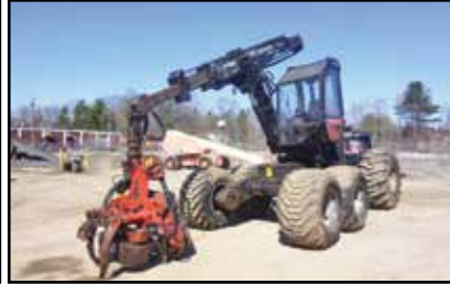
ITEM 8339 1999 VALMET 911C, FULL TREE HARVESTER, MD965 HEAD 28", 29' CRANAB BOOM, FULL COMPUTER MEASURING SYSTEM, A/C&HEAT. $59,500.00
