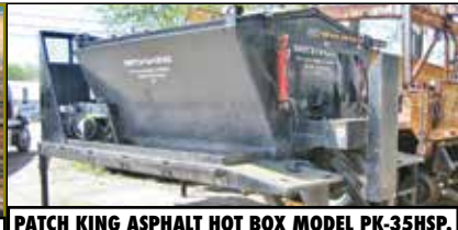
PATCH KING ASPHALT HOT BOX MODEL PK-35HSP. 3.5 yards, rotary auger, discharge chute & hyd. lids, 240 vt electric operated, stays warm 10 hours, tack tank & 6500 watt generator mounted on hook-lift frame, can be truck mounted, little use, 800-464-0573, www.WestsideTruckEquipment.com
