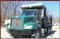
2012 KENWORTH T470 T/A DUMP TRUCK, Paccar PX-8 6 Cyl 8.3L Diesel 330 HP, Engine Brake, Eaton Fuller RTO 8LL Janual Trans, 18K FA, 46K RA, Dana Drive Axles, Double Fram Hendrickson Susp, Brandon 14' High Steel Body, Just Serviced \$79,900
