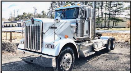
2016 KENWORTH W900L. 560 Cummins, 18 Spd., 13,200 Front, 40,000 Rears, Wet System, 593K, Motor Was Done At 407K, Truck Runs And Goes Great, \$79,000 OBRO. 207-229-2120
