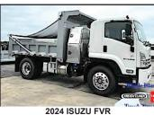
12' STEEL DUMP BODY, 152" WB, 33,000 GVW, 6.7L CUMMINS DIESEL. #RSB00342
