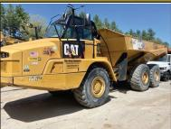
2014 CAT 730C, Rubber front 50% rear 25-30%,Tailgate, 8550 Hours, 6x6, Has Transmission Leak, Rear Tailgate,\$169,000. Runs Great!
