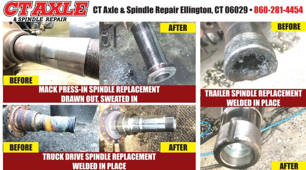
• Drive Spindles From 1 Ton To Class 8 Trucks • Trailer Spindles From 3,500# To Class 8 Axles Spindles can also be repaired by welding up the worn area and then remachining to factory spec.
