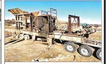
TELSMITH 30 X 42 JAW WITH MAGNET. Tri Axle Chassis, 36" Take Away Belt, New Jaw Dies, 4 X 20 Feeder, 150 Hp Motor, Call For More Information.
