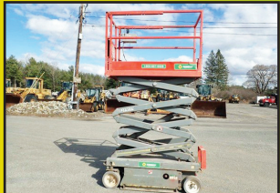
2012 SKYJACK SJIII3219: 147 Hours, 19 Ft Electric Scissor Lift, 32" Wide, 5 Ft Basket + 3 Ft Extension, stk#AE924, $6,500
