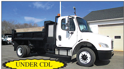
2007 FREIGHTLINER M2 : CAT C7-230HP, PRE-EMISS., 95K MILES, ALLISON 3500 RDS AUTO, 26K GVW, SPRING SUSP. LOCK DIFF., 5.38 GEARED RATIO, SINGLE FRAME, AIR-BRAKES, A/C, ELEC. PUMP, 10' STEEL DUMP, TOOL BOXES, TARP, PINTL. $37,000
