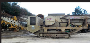
KOLBERG-PIONEER 2650 JAW CRUSHER TRACK-MOUNTED 26X50 JAW, SIDE DISCH CONV, MAGNET, HOPPER, NEW ENGINE, CHAINS & SPROCKETS $259,000
