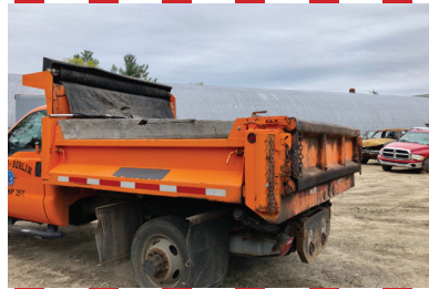
9' GALION DUMP BODY. Fold Down Sides, Central Hyd, Load Cover, DRW, Rock Solid, #NOF, $3,500
