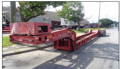
1987 LIDDELL-BIRMINGHAM 50 TON BEAM TRAILER , Tri Axle, Air Ride, Hydraulic Detachable Gooseneck, Self-Contained Power Unit, 28' Deck, 22.5 Rubber. Call For More Information.
