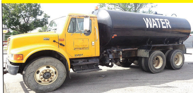
2001 INTERNATIONAL 4900 WATER TRUCK , 4,000 Gallon Tank, Front Rear And Side Air Operated Spray Heads, Spring Ride, Cummins 530 HP, 8 Speed, One Owner, Exc Shape, Tandem Axle, A/C, P/S, Call For More Information.
