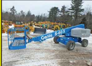
2011 GENIE S60X: 5,567 hours, 60 ft boom lift, 50 ft horizontal reach, 4x4, 8 ft basket, 4 cyl Perkins diesel, stk#AE253, $31,500
