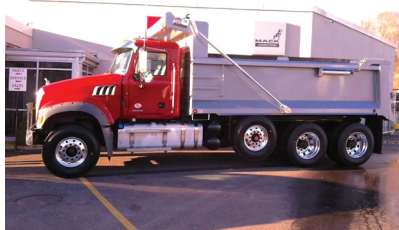
NEW 2019 MACK GRANITE 84FR: Heavy Duty MP8-425HP, Tri-Axle Dump, Fuller 8LL, 18 Front/46 Rear, 23,000# Pusher Axle, 176 Dump Body, 237" Frame, Call For Best Price !
