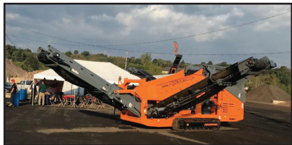
2017 ROCKSTER RSS410 SCREENER - 4'x10' Two Deck Scalping Screen, Punch Plate, Diesel Engine, Wired Remote Control - $159,000 CALL DAN AT 203-506-3860
