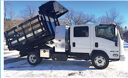
NEW 2019 ISUZU NRR: Medium Duty Isuzu Crew-Cab Landscape Truck, 19,500 GVW, 4HK1-TC, Diesel, Auto, 215HP., Leaf Spring Susp., 150"WB, 9'6" Rack Dump, All Steel Wheels And So Much More ! Call For Best Price !
