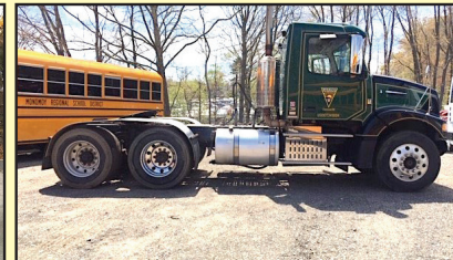
2013 VOLVO VHD64FT200-D13, 475HP, 8LL, 14,600 FRONT/46,000# REAR ON T-RIDE, WET-SYSTEM, 193,777 MILES. #180264A
