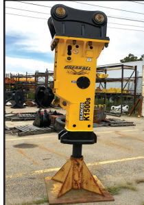
NEW BREAKALL K1500 HYDRAULIC HAMMER, Operating Weight 2,866 lbs., Impact Rate BPM 350-750, Tool Di- ameter 4.7", Impact Energy 3,500 lbs., Carrier Weight 31,000 - 42,000 lbs., Fits A 320 Excavator. $19,950 or $399/ Month. 401-785-9800
