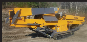
BARFORD TR8036 CONVEYOR 80'x36" TRACKED, TWIN DRIVE, HYD SLEW HUBS, HYD RAISE & LOWER, HYD HEAD FOLD, CAT 2.2 TURBO ENGINE, NEW! $99,000
