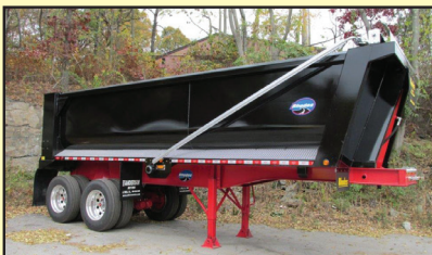
2020 RHODES 26' STEEL DUMP TRAILER AR450, DUAL HINGE HIGH LIFT-GATE, 70,000# SINGLE POINT, ELECTRIC COVER.
