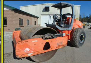
2010 HAMM 3410: 3,269 hours, 84" smooth single drum, drum drive & vib., 4 cyl Deutz turbo, 134 hp, orops, stk#CO286, $42,500
