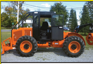
AWASSOS MD80. Log Skidder, 84HP, 12,000 lbs, Hydosttic Drive, Grapple, Winch, 7.5'-8.5' Wide
