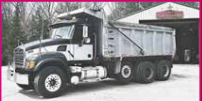
2006 MACK CV713. 427 Mack, 8LL, 18FA, 20LA, 44R on camel back, very good 17' steel body, perfect double frame, 220K, paving truck, $67,500.
