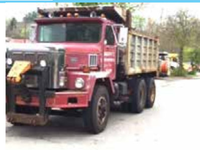
1998 IH PAYSTAR 205K MILES 315 CUMMINS 8LL TRANSMISSION 18K FRONT 46K REAR WALKING BEAM SUSPENSION 13 FT 6 INCH DUMP BODY 11 FT WING PLOW INCLUDED. A BIT RUSTY AND NEEDS A BIT OF TLC BUT AN OLDIE BUT GOODIE. SALE PRICE $15,500.00
