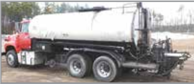
1990 FORD LTS9000 4175 GALLON TANDEM AXLE ASPHALT DISTRIBUTOR TRUCK. CUMMINS 350, ENGINE BRAKE, EATON FULLER 8LL, DOUBLE FRAME, HENDRICKSON SPRING SUSPENSION, 12,000 LB FRONT, 38,000 LB REARS, 208" WHEEL BASE, ALUM WHEELS, ETNYRE BT-HL DIST, 6' SPRAY BAR, 4' EXTENSIONS, IN CAB CONTROLS. CALL FOR MORE INFORMATION.
