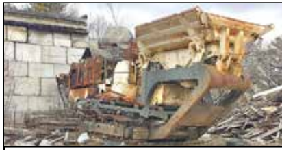
NORDBERG 80 CRUSHER. Motor burned along with the controls and the discharge belt. The jaw was not harmed by the fire. $15,000. 603-717-5137
