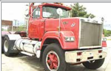
1987 MACK SUPERLINER RW713, 425 CAT, 8 SPEED, BRAKE SAVER, MACK CAMEL BACK SPRING, AIR RIDE CAB, 58K LB REAR, 20K FRONT, DOUBLE FRAME, WET SYSTEM, 12 X 2400 NEW GOODYEAR TIRES, 300K MILES, P/S, A/C, DUAL STACKS, HEAVY DUTY FIFTH WHEEL, ONE OWNER. EXCELLENT CONDITION. CALL FOR MORE INFORMATION.
