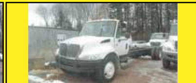
2004 IH 4300 Cab & Chassis. DT466, 6 speed, 154K miles, hyd brakes, 254" WB, 186" CA, low miles, $12,995
