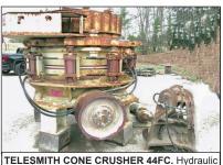
Adjust With Hydraulic Tank And Lube System.
