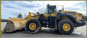
2020 KOMATSU WA500-8 A/C, 8CY BKT, 353HP TIER-4 FINAL DSL, 4-SPD PWRSHFT TRANS, RIDE CTRL, FCTY ON-BOARD SCALE, REAR CAM, NEW 29.5R25 L3 RADIALS, 2540 HRS \$219,000
