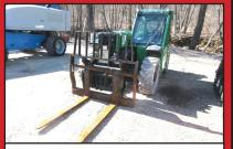
2015 JLG G5-18A TELEHANDLER, Just Serviced & Ready To Go. Enclosed Cab, 18' Max Lift Height, 5500 lb Max Lift Capacity, 48" Forks, Manual Coupler, Auxiliary Hydraulic Plumbing, 33 x12-20 Aperture Tires, Green, \$38,900
