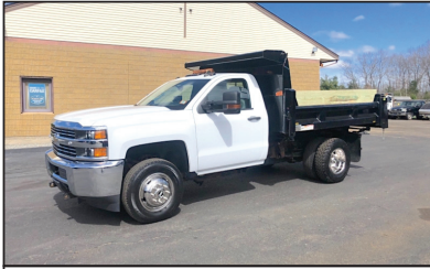
2017 CHEVY SILVERADO 3500HD. 4WD, Fisher Stainless Steel V-Plow, 28K MILES, Gas 360 Hp, Auto, 9' Dump Body, Remainder Factory Warranty, $44,490.
