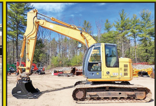
2008 JOHN DEERE 135C RTS: 6,339 Hours, 39" Bucket, Hydraulic Coupler, 1-Way Aux. Hydraulics, A/C, Reduced Tail Swing, 4 Cyl Isuzu Turbo, 90 HP, 31K Lbs, stk#XC890, $52,500
