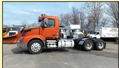
2016 VOLVO VNL64T300-D13, 500HP, 18SPD., 14,600 FRONT/46,000 REARS, AIR-RIDE, 2 LINE WET-SYSTEM.
