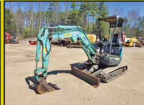
2014 IHI 25VX3: 1,573 Hrs, 12" Digging Bucket w/New Teeth, 2 Way Aux. Hydraulics, 2 Spd Travel, Control Pattern Selector, 0 Tail Swing, Good Rubber Tracks, Blade, Swing Boom, Yanmar Diesel, 6.1K Lbs, stk#MX532, $22,500
