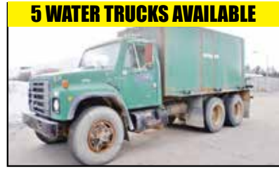
1984 INTERNATIONAL F1954 4000 GALLON TANDEM AXLE WATER TRUCK, 210 HP, EATON FULLER 13 SPEED, HENDRICKSON RT SERIES SUSPENSION, 10,860 LB FRONT, 38,000 LB REARS, 170 INCH WHEEL BASE, PORTA-TANK PTAC-21 TANK, WACKER PT3A PUMP, REAR SPRAY, CALL FOR MORE INFORMATION.
