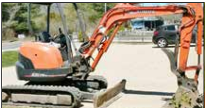
2007 KUBOTA U35 SUPER SERIES. Hyd. thumb, quick change bucket, 8000lb. machine, 2360 Hrs., new tracks and sprockets at 2000 Hrs., $25,500. Charlestown, RI 401-788-4212
