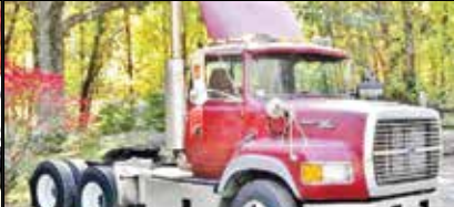
1995 FORD L9000 . CAT 3176, 365 HP, 10 speed, Jake brake, locking rear end, 213,249 miles. Asking $18,500 OBO. Ludlow, MA 413-547-6082
