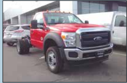
2016 Ford F550 XLT Chassis Cab. 6.7L diesel, 4x4, #160062
