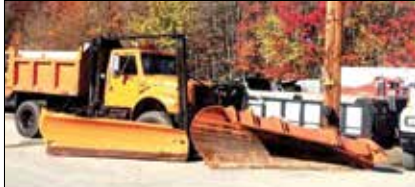
1995 INTERNATIONAL 4800 , All Wheel Drive, 12x25.5 virgin tires, DT466 mechanical, Fuller 6 spd, front & wing plow set-up, call for more details, $22,500., Lunenburg, MA 866-377-8729
