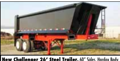
New Challenger 26' Steel Trailer, 60" Sides, Hardox Body, Hi-Lift Tail Gate, 2-Speed landing Gear, Tapered Nose, 60K Single Point Suspension, 25K axles, LED Lights, 4 Wheel ABS, 24.5 16ply tires, Hub Piloted Steel wheels, $53,350.00 Includes FET, Consolidated Truck & Equipment, Rehoboth, MA, 508-252-3339
