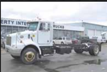
1996 PETERBILT 330 C&C, 8.6 CUMMINS DIESEL, 10 SPD, AIR RIDE, AIR BRAKES, 256" WB, TRAILER PKG, 31K GVW, 437K MILES, STK#10528
