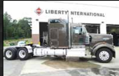
2009 KENWORTH W900 72" SLEEPER 6X4, ISX CUMMINS 485HP DIESEL 13 SPD OD, ENGINE BRAKE, AIR RIDE, T/A, 59,200 GVW, 322K MILES, STK#10151
