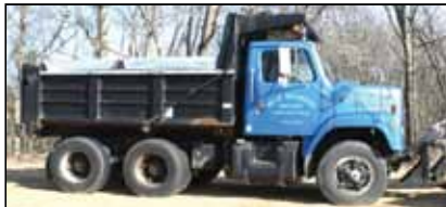
1986 International. 350 Cummins, Jake 7-speed, heated 12' body, 20K miles on clutch & brakes, new dump cyl., legal 15 tons, 85K on inframe. Don't need any more; good truck for the money, $14,500. Suffield, CT 860-798-6680
