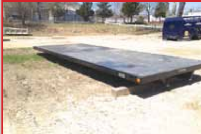
Heavy Duty 22' Platform Body 102" wide, 10" long sills, 12" o/c cross members, 3/16" smooth steel floor, $5,300
