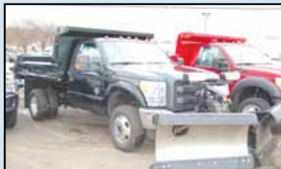
2012 Ford F350, diesel, power group, 2/3 yard dump, double acting hoist, 9.5' Fisher Stainless V Plow, alum wheels, #120445
