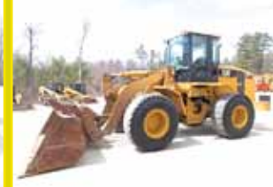
1999 CAT 938G: 3.65 YD, BALDERSON HYD CPLR W/ 3RD VALVE, 6 CYL CAT TURBO, A/C, 29K LBS, STK#0402, $51,500
