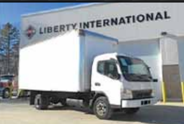
2006 MITSUBISHI FUSO FE180 18' SUPREME VAN, 4 CYL 175HP DIESEL, AUTO, ENGINE BRAKE, SPRING, E-TRACK, 90" H X 96" W, 17,995 GVW, 190K MILES, STK#10442
