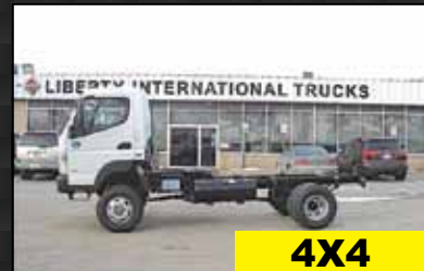
NEW 2012 MITSUBISHI FUSO FG140 4X4 C&C, 4 CYL. 160HP DIESEL, AUTO OD, SPRING, 134" WB, 14,050 GVW, STK#M1174
