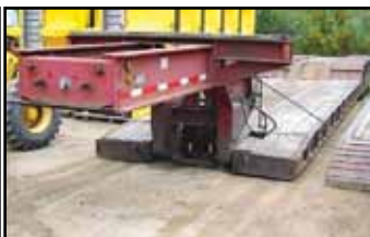
1988 ROGERS 50-TON LOW BED TRAILER, 102" wide, 22' deck, covered rears, walking beam suspension, 10 outriggers per side, Stk#UT1204, $20,000
