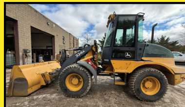
2017 DEERE 324K CAB, A/C, 3 RD VLV AUX HYD, 88" GP BKT, RIDE CTRL, 405/70R20 RADIALS, 2,303 HRS $69,000
