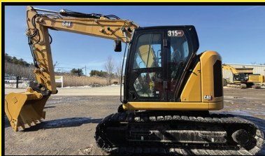
2023 CAT 315GC A/C, 8'2" STK, AUX HYD, HYD Q/C, 36" CAT BKT, ENG TURBO, GRD CTRL, PTRN CHNGR, 20" RBR PADS, 1,594 HRS $142,500
