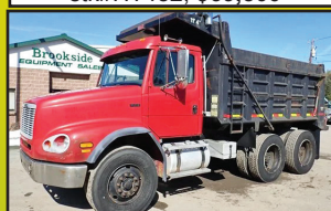
2003 FREIGHTLINER FL112Z: 377,047 Miles, 10 Wheel, 13'6" Steel Bibeau Body W/ 3 Chutes, Cat C12, 430 Hp, Fuller 8LL, 18k F, 46k R, Hitch, Spring Suspension, stk#TK065, $37,500
