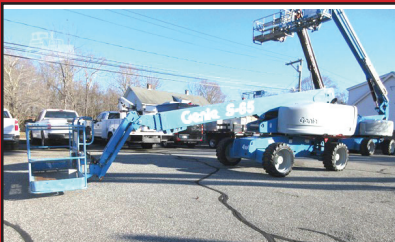
2014 GENIE S-65, 65' Max Platform Height, 500 lb Max Weight Capacity, Jib, Power To Platform, Perkins 4 Cylinder 2.2 L Diesel Engine, 355/55D625 Tires $26,500
