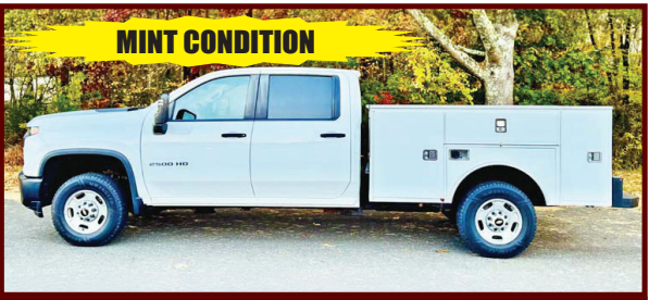
2022 CHEVY C2500 CREW CAB 8' UTILITY. 6.6L V8, Auto, AC, Rear Camera, Bluetooth, 6-Passenger, Southern Truck, 110K, Fleet Maintained, $34,400.
