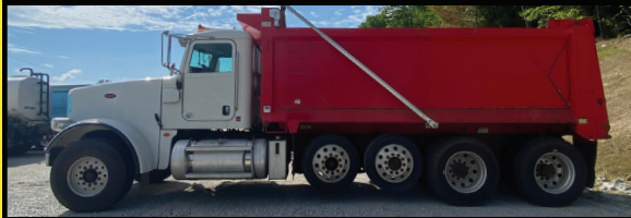
2015 PETERBILT 367 10X4, A/C, 485HP PACCAR MX-13 6CYL, ENG BRAKE, EF AUTO, DIFF LOCK, 4.10:1 RATIO, 80K LB GVWR, 425/65R22.5 F & 11R24.5 R TIRES, STEERABLE AIR LIFT TAG AXLE, DUAL STR BOXES, DBL FRM, HENDRICKSON HAULMAXX, 254" WB, 18'L X 5'H HERITAGE STEEL BODY, ELEC ROLL TARP, HI-LIFT TAILGATE, 180K MI $99,000
