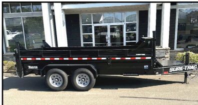
SURE-TRAC 15.4K PRO SERIES TELESCOPIC DUMP TRAILER. 7' x 14', Heavy Duty I-Beam Frame And Tongue, #454378
