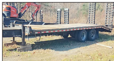
2020 KAUFMANN 25K TRAILER. DUAL TANDEM, ELECTRIC BRAKE, EXT RAMPs, SPARE, $9,350.
