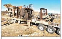
TELSMITH 30 X 42 JAW WITH MAGNET. Tri Axle Chassis, 36" Take Away Belt, New Jaw Dies, 4 X 20 Feeder, 150 Hp Motor, Call For More Information.
