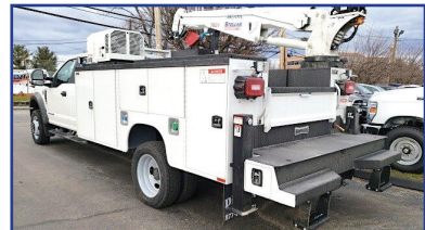
2019 F550 KMT MECHANICS BODY. Stellar 7,500lb Crane, Out Riggers, Air Compressor, Diesel, 4WD, Power Equip Group, Payload Upgrade, FN1374
