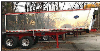
2020 RHODES. 26' Aluminum Double Walled Smooth Side Dump Trailer, Steel Frame, 70,000# Single Point. Call 401-434-5900
