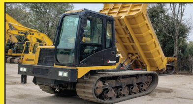
MOROOKA MST2200VDS A/C, 250HP CAT DIESEL, HST TRANS, 12' DUMP BODY, 30" RUBBER TRACKS, 30,000LB CPTY STARTING AT $89,000
