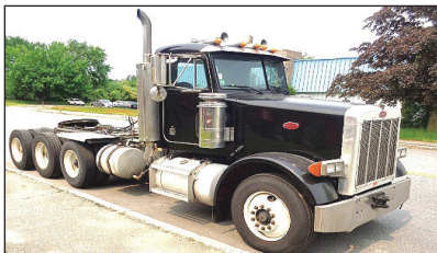
1996 PETERBILT TRACTOR , Tri Axle, CAT Power, 8 Speed, 46K Rears, 20K Pusher, Wet System, Pintle Plate, 24.5 Rubber, Long Enough For Dump Body, Air Ride, Call For More Information.
