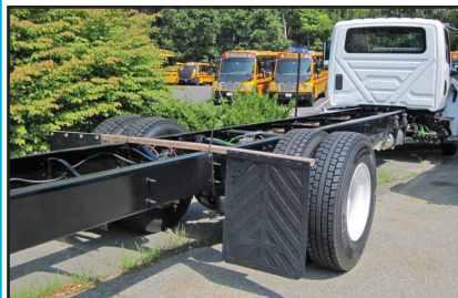
2025 INTERNATIONAL MV607. Under CDL (25,999 GVWR) With Air Brakes, Cummins 6.7 250HP W/ Allison 2500 RDS 6 Speed, A/C, PW, PL, Air Ride Suspension, Air Driver With 2 Man Passenger, 11.25 Hankook Tires, We Will Shorten Wheelbase If Needed
