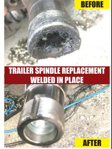
• Drive Spindles From 1 Ton To Class 8 Trucks • Trailer Spindles From 3,500# To Class 8 Axles Spindles can also be repaired by welding up the worn area and then remachining to factory spec. This includes tracing threads or remachining new threads.
