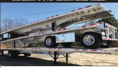
Crossmembers On 18" Centers, 3 Wood Nail Strips, King Pin Set At 30", Fixed Spread Axle, Air Ride Suspension, Lock-Rite Side Rail With Stake Pockets, Sliding Winches, Aluminum Air Tank, Tool Boxes, Call For Complete Details, 207-274-3525
