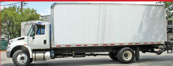
2017 INTERNATIONAL DURASTAR 4300 26' VAN. 102" X 102", Allison Auto, AC, Air Ride Suspension, Non CDL, 4300 LB Alum. Lift Gate, 223K Miles.
