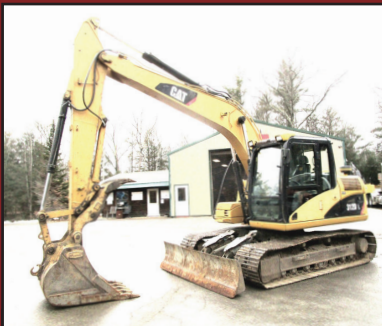
2008 CAT 312DL. 6040 Hrs, Long Stick, 36" Bucket, 24" Shoes, CAT Full Rotation Thumb, Aux. Hyd., 8'6" Blade, Legal Width, $89,000.
