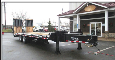
CAM SUPERLINE 20 TON HD DECKOVER. 8' 6" x 27', 22' Flat + 5' Beavertail, 40" x 80" Air Ramps With 36" Extension, #525644
