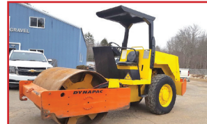
1989 DYNAPAC CA151-1D. Vibratory Compactor, 3,867 Hours, 66" Smooth Drum, #2657, $29,500
