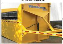
**VIBROSCREEN SCM-75** HEAVY DUTY SCREENER Vibrating Head w/2 Decks , Up to 300 Cubic Yards/ Hour, 50 HP Diesel Engine, ldeal For 6 Yard Loader, Fifth Wheel Hitch, Single Axle, Double Wheels, Hydraulic anding Gear, Gross Weight 22,000 LBS Tongue Weight 8,540 LBS Rental Rates:
