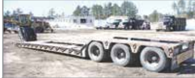
2007 TALBERT 55 TON TRI AXLE LOWBOY, AIR RIDE, HYDRAULIC DETACH NECK, NON GROUND BEARING, 102" WIDE, 25' 6" DECK. COVERED BOGIE. CALL FOR MORE INFORMATION.
