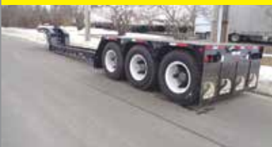
1989 TRAIL KING 65 TON BEAM TRAILER, 24' BEAM, 3 AXLES, SPRING RIDE, NON GROUND BEARING, 8' 6" WIDE, LONG GOOSENECK, 12 X 24 RADIAL TIRES. SANDBLASTED AND PAINTED, NEW BRAKES, SEALS, HUBCAPS, DECALS AND FLAPS. EX-NYC TRAILER, LIKE NEW CONDITION. CALL FOR MORE INFORMATION.
