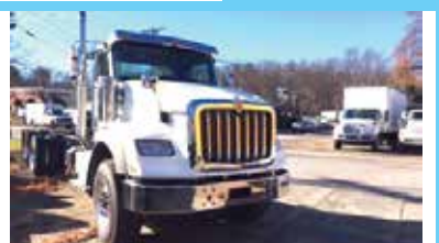
2017 INTERNATIONAL HX THE BEST VOCATIONAL TRUCK BUILT. 455 CUMMINS, HENDRICKSON PRIMAXX AIR RIDE 46 RR 20K FRT. 8LL 2 PEDAL ULTRASHIFT TRANSMISSION. LONG WB
