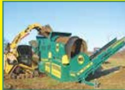
New REVOLVER 508 TROMMEL SCREEN : With Rear discharge Conveyor, Cat Diesel, 5' x 8' Quick change drum, Reversible rotation 4-1/2 Cu.Yd. hopper, 8' dump height /load with skid steer, Hydraulic legs for hook-up
