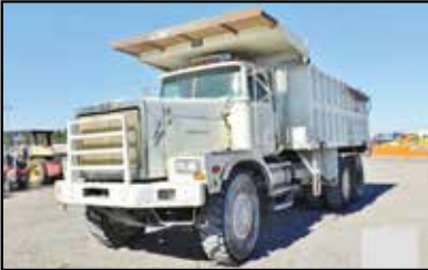
2007 WESTERN STAR 6900XD OFF ROAD TRUCK, DETROIT SERIES 60 12.7L, 445 HP, ENGINE BRAKE ALLISON AUTOMATIC TRANSMISSION, DOUBLE FRAME, BEAM SUSPENSION, 28,000 LB FRONT, 100,800 LB REARS, AXLETECH PLANETARIES, 230 IN WHEELBASE, 11' WIDE, 33' 8" LONG, 12' 8" HIGH, PTO, J & J 20' BOX, 14.00 X R25 TIRES. CALL FOR MORE INFORMATION.
