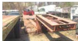
1972 Schertzer 75 Ton Detachable Low Boy w/ drop sides, 33' steel deck, 15' tail, 60' total length, 10' wide, excellent cond, A Steal @ $18,950/OBO
