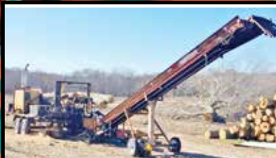
BRUTE FIREWOOD PROCESSOR. 4 CYL JOHN DEERE, 24" HYD CHAINSAW, 4 OR 6-WAY HYD SPLITTING WEDGE, 2-STRAND LIVE DECK, 20' TIMBERWOLF BELT CONVEYOR, 5.5HP HONDA ENGINE, $21,500. 617-839-8880
