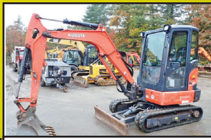
2019 KUBOTA KX033-4: 4,200 Hours, 24" Bucket, Cab W/ A/C, Auxiliary Hydraulics, Manual Coupler, 61" Blade, 2 Speed, 3 Cyl Kubota D1703, 7.8K Lbs, stk#MX122, $29,900
