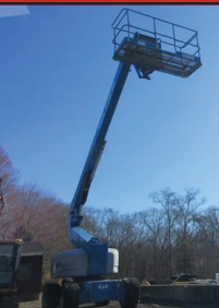
2015 GENIE Z80/60 ARTICULATING BOOM LIFT. 78' Max Platform Height, 500 lb Max Weight, Jib, Power To Platform, Onboard generator, Deutz 2.9 L4 4 cylinder 74 HP Diesel, Foam Filled Tires. Freshly Serviced & Safety Checked. $35,900
