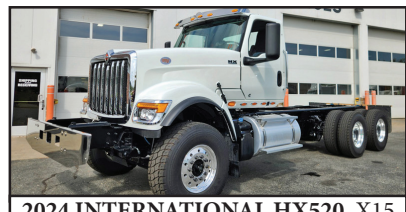
2024 INTERNATIONAL HX520. X15 Cummins, Allison Auto 4500, 20/46 Axles, Air Ride, Aluminum Wheels, Ready For A Dump Body
