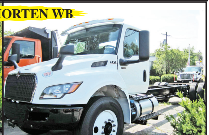
2025 INTERNATIONAL MV607. Under CDL (25,999 GVWR) With Air Brakes, Cummins 6.7 250HP W/ Allison 2500 RDS 6 Speed, A/C, PW, PL, Air Ride Suspension, Air Driver With 2 Man Passenger, 11.1R 225 Hankook Tires, We Will Shorten Wheelbase If Needed
