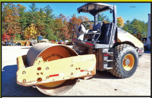
2014 VOLVO SD115: 5,716 Hours, 84" Smooth Single Drum, Drum Drive, Vibratory, Drops, 4 Cyl Volvo Turbo, 148 HP, 26K Lbs, stk#CO067, $39,500
