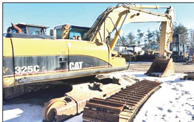
2003 CATERPILLAR 325CL. Plumbed For Hammer, Quick Disconnect, Working Daily, Needs A Final Drive. Call For More Information.
