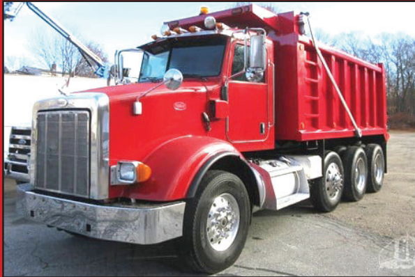
2011 PETERBILT 365 TRI-AXLE 6x4 DUMP. Cat C13, 6 Cylinder 12.5L Diesel 335 HP, Engine Brake, Allison Auto, 16540 FA, 59500 RA, Air Ride, Steerable Air Lift Pusher Axle, Double Frame, Wet Kit, $115,000
