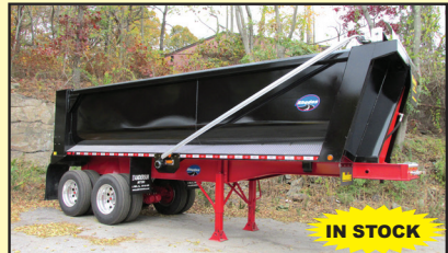
IN STOCK 2024 RHODES RSS2660-2 26' STEEL END DUMP TRAILER, AIR HIGH-LIFT DOUBLE ACTING TAIL GATE, HD SPECS.
