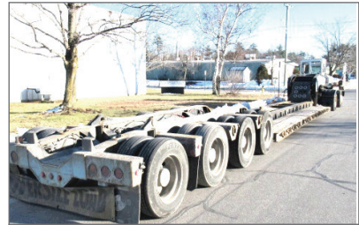
2016 FONTAINE MAG60 DSR. 28' Deck, 3 Axles With Pin On 4th, 2 Lift Axles, 60" Axle Spacings, Set Up For Gooseneck Extension To 183", One Owner, Original Paint, Call For More Information.
