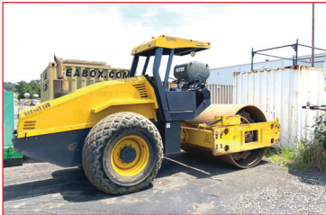
2008 BOMAG BW213DH-40 84" SMOOTH DRUM, VIBRATORY, 13 TON. 4,500 HRS. STK# R-60
