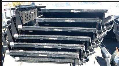
EZ DUMPER. New Slide-In Dump Body, Complete Head Board, Tarp, & Hoist. 603-483-2541
