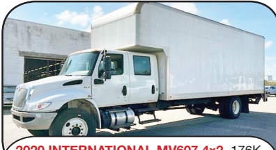
2020 INTERNATIONAL MV607 4x2 , 176K, Cummins B6.7, Allison 2100HS 6sp Auto, Crew Cab, 24' Attic Peak Box, 3300 Lb Tuckaway Liftgate, Ready For Moving Season! stk#202566, $79,900.
