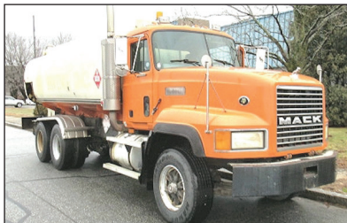
1996 MACK CL 713, 350 MACK. 13 Speed Mack, 46K Rears, 4,100 Gallon Two Compartment Tank, Remtec Inc Steel Tank, 1100 X 24.5 Rubber, 270,000 Original Miles. Call For More Information.
