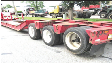
2003 TALBERT 50 TON 9 WIDE TRI AXLE PAVER STYLE TRAILER. Non-Ground Bearing, Three Axle, Air Ride, Lift On Third, 25 1/2 Foot Long Lower Deck, 5 Foot Slope, Covered Back, Excellent Shape, One Owner, Call For More Information.
