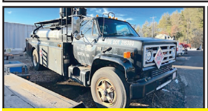
Site Or Storage * Fast Flow 1985 GMC Liquid Test Measurement Truck. Detroit, 5+2 Trans, 1500/500 Gal Compts Testing Top & Bottom All Liquids, 3" Pump, Good Cond. $15,000
