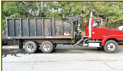
2000 VOLVO WG64B, 275HP. AUTO, 16,000# FRONT / 40,000# REARS, JOHNSEER 820 CRANE, 20' DUMP BODY. #210299A
