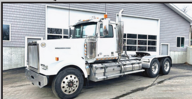
2018 WESTERN STAR 4900EX. DETROIT DD16 600 HP, EATON 18 SP ULTRASHIFT, 235" WB, NEW 24.5 TIRES, 46K REARS, 14.6K FRT, 330K MILES, 2 LINE WET SYSTEM, FACTORY STROBE PKG & LOWBED SERVICE, LIGHT & GAUGE PKG, $104,000. SAUGUS, MA 781-307-3243
