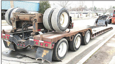
2012 55 TON FONTAINE. (2 Available To Choose From 2009 And 2012), Tri Axle With Pin On 4 Axle, 25 Foot Deck, Powerpack, Full Fenders, Air Ride, Texas Trailer—Rust Free, Call For More Information.
