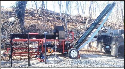
FIREWOOD PROCESSOR. Fully Hydraulically Automated, All One Unit, 35 HP Gas Engine, 15' Conveyor, Can Be Brought Up And Down, Splitter Blade, 6-Way Can Be Hydraulically Moved Up Or Down, Hydraulic Chainsaw, 25" Bar, Indeed Conveyor, Chain Driven Log Table, Custom Built, \$15,000. 401-390-4976
