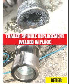
TRUCK DRIVE SPINDLE REPLACEMENT WELDED IN PLACE
