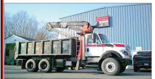
**2009 IH 7600 T/A DUMP LOG LOADER. Prentice** 120, Rotating Grapple, 22' Reach, Cummins 400PH, 8LL, Double Frame, 256K Miles, \$55,000
