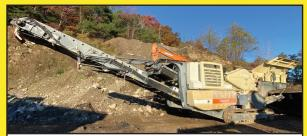
2016 METSO LOKOTRACK LT106 42"X28" JAW, CAT DSL, OVERBAND MAGNET, REMOTE CTRL, TRACKED, NEW JAW DYES, NEW FEEDER BEARINGS, 4761 HRS \$285,500
