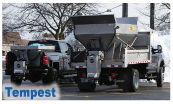
Available in chain drive or with the new Helixx shaftless auger system
