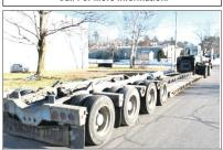
2016 FONTAINE MAG60 DSR. 28' Deck, 3 Axles With Pin On 4th, 2 Lift Axles, 60" Axle Spacings, Set Up For Gooseneck Extension To 183", One Owner, Original Paint, Call For More Information.
