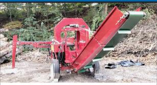
FIREWOOD PROCESSOR. FULLY AUTOMATED, 3 STRAND LOG TABLE, IN-FEED CONVEYOR, HYDRAULIC CHAINSAW 25" BAR, 4 WAY SPLIT BLADE (6 WAY AVAILABLE), OUT-FEED CONVEYOR, 30 TON FORCE, 27 HP MOTOR, 32 GPM PUMP, \$14,500. 401-363-1539
