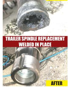
• Drive Spindles From 1 Ton To Class 8 Trucks • Trailer Spindles From 3,500# To Class 8 Axles Spindles can also be repaired by welding up the worn area and then remachining to factory spec.
