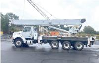
2006 ALTEC AC35-127S. 38 Ton, 127' Boom 31' Jib, Two Person Basket, Cordless Remote Control, Sits On 2006 Sterling L7500 Tir Axle, Mercedes OM460LA Diesel 455 Hp, Jake Brake, New Tires, 38,000 Miles, 5,364 Hours, Excellent Condition, \$125,000
