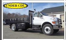
2012 FORD F-650: CUMMINS ISB-260HP, 119K MILES, ALLISON 3500RDS AUTO, 26K GVW, SPRING SUSP, SINGLE FRAME, 11R 22.5 TIRES, AIR-BRAKES, A/C, PTO, 16' STEEL DUMP, BARN DOORS, TARP, PINTLE, AIR-TO-REAR. \$50,000
