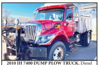
2010 H7 /400 DOMP PLOW TRUCK: Diesel 310 Hp, Automatic, 40,000 GVW, Swenson SS All Season Body, Aero Electric Tarp, Pintle Plate 24,040 Miles. Clean, MA State Inspected, Serviced #597109 \$42.500.
