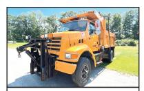
**2000 STERLING L7500.** 3126B CAT, Spicer 7 Speed, Spring Susp, 4.56 Ratio, 11R22.5, Highway Plow, Steel Dump Body, 73,080 Miles, #F34819, **\$13,500**
