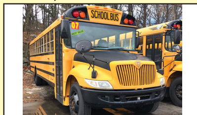
2007 INTERNATIONAL IC, 77 PASSENGER SCHOOL BUS, DIESEL, AUTO, HYD. BRAKES. #180147A
