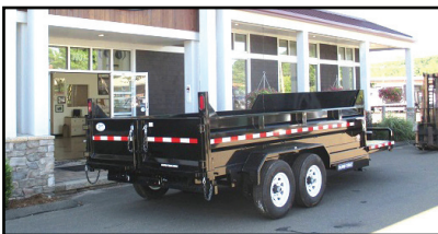
SURE-TRAC 14K DUMP TRAILER. 6' 10" x 14' + 4' Stationary Deck, Tandem Axle, #K2252738
