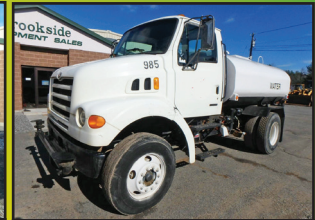
1999 Sterling L7501: 10,579 miles, 6 wheel water truck, 2000 gallon, Cat 3126, 330 hp, 6 speed, 12k f, 19k r, spring suspension, stk#TK736, $27,500
