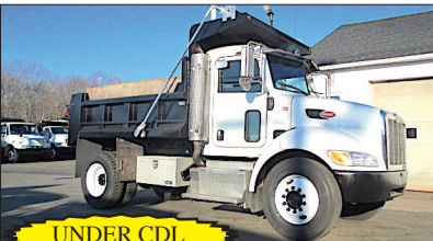
2013 PETERBILT 337 : PACCAR 220HP, 88K MILES, ALLISON AUTO, 26K GVW, SPRING SUSP. W/ HELPERS, LOCK DIFF., SINGLE FRAME, HYD. BRAKES, AIR-SEAT, A/C, PTO, NEW 10" STEEL GALION DUMP, AUTO TARP, PINTLE REC., RARE TRUCK ! $59,000
