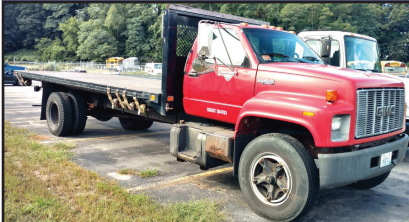
1995 GMC TOPKICK 7000. 6 Cyl. CAT Diesel Power 3116, 6 Speed Standard, 22' Flatbed, 224,400 Miles, 25,950 GVW, Asking $5500. Woonsocket, RI 401-769-0271
