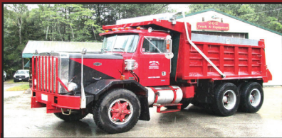
1987 AUTOCAR DK64. 350 CAT 3406B, 8LL, 20F + 58R, Very Good 12R24 Tires, New Clutch, 14' Steel Body, Factory A/C Everything Intact But Not Working, 5.29 Ratio, DOT Good, $27,000.
