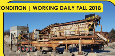
CEDARAPIDS CSC380MVP6203 CLOSED CIRCUIT CONE PLANT, 4 AXLE CARRIER, 6x20 2-DECK SCREEN $195,000
