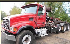
2004 MACK GRANITE TRI-AXLE W/ AMERICAN 75,000LB 22' HOIST RE-MACK TRANS., NEW CLUTCH, REBUILT PTO, NEW HYD. PUMP, PIONEER COVERING SYSTEM, NO PINTLE, 541K MILES. $45,000
