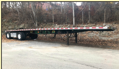
2013 FONTAINE 48 X 102 ALUMINUM DECK ON STEEL FRAME, AIR-RIDE, 10'2 SPREAD AXLE, NEW TIRES & BRAKES.
