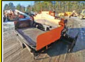
2003 LeeBoy L700ST: 1,997 hours, 8-12 ft tracked paver, 2 cyl Hatz diesel, stk#PA43B, $22,500
