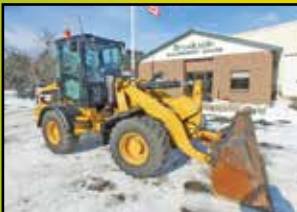
2012 Caterpillar 908H2: 2,629 hours, 1.4 yard, hyd coupler w/ 3rd valve, cab, 4 cyl Cat turbo, forks, 2 speed, 14.5k lb size class, stk#LO530, $57,500
