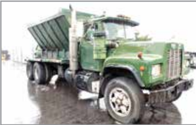
1990 MACK RD688 TANDEM AXLE ASPHALT SPREADER TRUCK , E7, 400 Hp, Eaton Fuller 8L, Double Frame, 18,000 Lb Front, 46,000 Lb Rears, Camel Back Spring Susp, 234" Wheel Base, Pto, Body Is 18' Overall Length, Bergkamp 14" (Hopper) Spreader Box, 24" Belt, Engine Brake, 11 X 24.5 Rubber, P/S, A/C, Truck From Florida, No Rust. Call For More Information.
