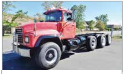
1999 MACK RD688S CAB & CHASSIS , E-7 350, 350 Hp, Engine Brake, Maxitorque, 13 Speed, Air Lift 3Rd Axle, Double Frame, Wet System, Camel Back Spring, 18,000 Lb Front, 44,000 Lb Rears, 226 Inch Wheelbase, Frame Recently Sandblasted And Painted, Set Up For 17' Dump Body. Call For More Information.
