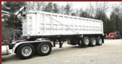
1996 SPECTEC 32' TRI-AXLE END DUMP. Very Good Liner, Forward Lift Axle, 66" Sides, 2-Way Gate, 6 New Alum. Wheels, New Springs & Bushings, $22,500.
