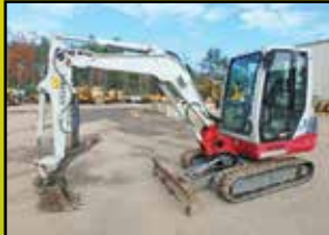
2011 Takeuchi TB235: 1,521 hours, 18" bucket, 64" blade, hydraulic thumb, manual coupler, cab w/ a/c, 3 cyl Kubota, 2 speed, 8k lb size, stk#MX988, $29,500
