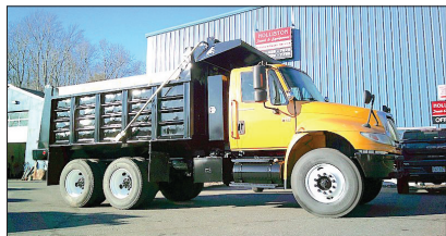
2006 INTERNATIONAL DUMP. DT466 300 HP, Automatic, 48K Miles, Double Frame, 14' Steel Body, 3 Chutes, 56,000 GVW, Air To Rear, Pintle, $53,000
