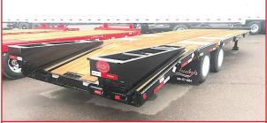
2024 FELLING FT 40. 20' deck, 6' Double incline Beavertail, 30" Spring Assisted Ramps, 16 D Rings, Oak Decking , A Frame Tool Box, Black Paint
