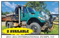
HP, Allison, 16 F/A, 30 R/A, Locker Tenco Plow Equipment Rev Blade And Wing Included.
