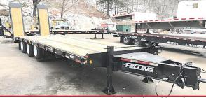
**2024 FELLING FT 45 2-LP.** 20' deck, 6' Double incline Beavertail, 30" Air Assisted Ramps, 235/70/17.5 Tires, 16 D Rings, Oak Decking, A Frame Tool Box, Black Paint
