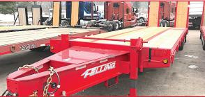
**2024 FELLING FT 45.** 24' deck, 6' Double incline Beavertail, 30" Air Assisted Ramps, 16 D Rings, Oak Decking, A Frame Tool Box, Red Paint
