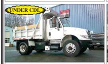
2011 INTERNATIONAL 4300, DT466-250HP., 120K MILES, EXHAUST BRAKE, ALLISON 3500RDS AUTO, 26K GVW, SPRING SUSP., SINGLE FRAME, AIR-BRAKES, PTO, 10' ALUM. DUMP, 1 CHUTE, AIR-GATE AND MORE 1 \$40,000
