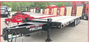
2024 FELLING FT 50. Air Tilt, Air Ramp, 24' deck, 6' Double incline Beavertail, 8" Ramps Air Assist, 16 D Rings, Oak Decking, 3rd Lift Axle, A Frame Tool Box, Black Paint
