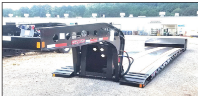
IN STOCK - NO WAITING - 2020 FONTAINE RENEGADE LXLN12 -12 Inch Loaded Deck Height With 4 Inch Ground Clearance When Fully Loaded, 30 Tons In 16 Feet On Tandem Bogie Or 30 Tons In 20 Feet With 3rd Axle Flip, Low Profile, 3rd Axle Capability, 32 Feet 11 Clear Deck Length. CALL FOR MORE INFORMATION.
