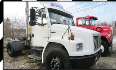
2002 FREIGHTLINER FL80: CAT 3126 330 HP, 95K Miles. Former Driving School Training Truck. Well maintained. Installing New Dump Body W/ Hitch Plate, D Ring, Air to Rear. Cover. Will paint your color. Call for Details & Price.
