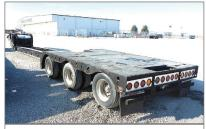
2005 XL SPECIALIZED 40 TON TRI AXLE BEAM TRAILER, Air Ride, 9' Detachable Neck, Self-Contained Power Unit, 25' Beam Deck, 102" Wide. Call For More Information.
