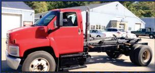
2007 GMC 7500 W/ NEW 18,500lb. Hook lift with 36" to 54" adjustable Jib. New Poly Fenders. New bumper & hitch.
