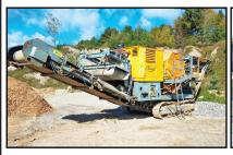
8784 2004 ERIN 1265J 49x26 TRACKED JAW CRUSHER. CAT C9 POWER, 12'-5"X 7'-7" FEED HOPPER, HYD MAGNET, 47" DISCHARGE BELT, 25" SIDE DISCHARGE BELT, \$125,000.
