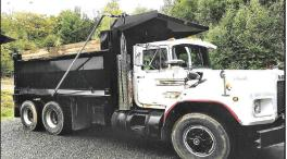
1991 MACK RB 688S E7, 350, 8LL, 18 Frt, 44 Rears, 2006 Beau-Roc Box Mounted In 2016, New Hinge, Hoist, Pump, & Tarp, Air & New Hook In Back,
