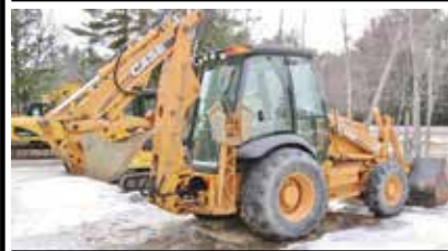
2008 CASE 580SM. E-Hoe, 4x4, Hyd. Front Q/C, Ride control, pilot controls, HYD. THUMB, 3000 hours, $37,500.
