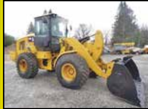
2013 CATERPILLAR 930K: 8,524 HOURS, 3.5 YARD, CAB W/ A/C, HYD COUPLER W/ 3RD VALVE, 6 CYL CAT TURBO, 31K LB SIZE CLASS, STK#LO143, $84,500
