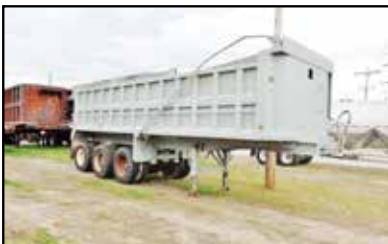
1999 J & J 30' STEEL TUB/STEEL FRAME TRI AXLE DUMP, SINGLE POINT SUSPENSION, AIR LIFT THIRD, 2 WAY GATE, FLIP N' GO CANVAS, RECENT SANDBLAST & PAINT. VERY GOOD CONDITION. CALL FOR MORE INFORMATION.
