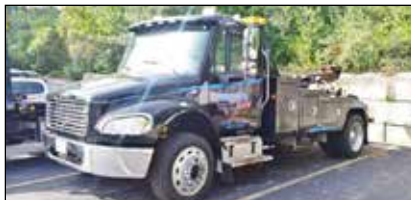
MEDIUM DUTY TOW TRUCK. Mercedes Benz motor & smart shift auto trans, Vulcan 897 14 ton body, stainless steel boxes, air brakes & air ride cab, 29,000 GVW, $25,000 OBO. 401-783-5979
