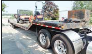
2002 FONTAINE HT35 HYD TAIL TRAILER, 48' X 102" WIDE, 2 AXLE, SPRING RIDE, BEAVER TAIL, WINCH, TOOL BOXES, ONE OWNER, ORIGINAL PAINT. CALL FOR MORE INFORMATION.
