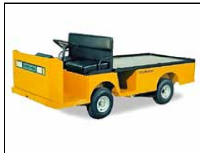
2016 TAYLOR-DUNN B-210 EE. 36-volt GT Electric Drive system, On-Board Automatic Charger, Headlights, Taillights, and Hydraulic Brakes
