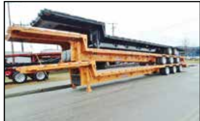
NEW 2016 DORSEY 53' TRI AXLE EXTENDABLE 50 TON STEP DECK TRAILERS, (2 AVAILABLE) AIR RIDE, 102" WIDE, 17.5 RUBBER. CALL FOR MORE INFORMATION.
