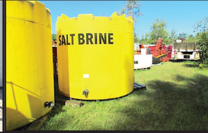
HIGHWAY SALT BRINE PRODUCTION UNIT. W/3000 Gallon Tank
