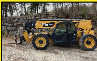
2020 CAT TL1255 12,000LB CPTY, 55' HT, EROPS, A/C, 60" FORKS W/ 72" CARRIAGE, FRONT OUTRIGGERS, 4,007 HRS $109,000
