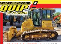
2018 KOMATSU D39PX-24 A/C, 10'8" 6-WAY PAT BLADE, JYSTK CTRLS, REAR CAM, 28" PADS, 4727 HRS \$69,000
