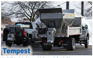
Available in chain drive or with the new Helixx shaftless auger system
