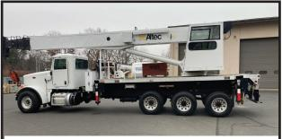
2013 ALTEC AC 38-127S. 38 TON, 127' BOOM, 31-55' JIB, BASKET, CORDLESS REMOTE CONTROL AVAILABLE, SITS ON 2013 PETERBILT TRI-AXLE, CUMMINS 380 HP, 10 SPEED, JAKE BRAKE, 23,384 MILES, 5383 HOURS, VERY GOOD TIRES, NO RUST, GO TO WORK CONDITION, OPERATOR CAB AVAILABLE \$175,000. 860-628-1771
