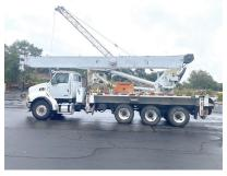
2006 ALTEC AC35-127S. 38 Ton, 127' Boom 31' Jib, Two Person Basket, Cordless Remote Control, Sits On 2006 Sterling L7500 Tir Axle, Mercedes OM460LA Diesel 455 Hp, Jake Brake, New Tires, 38,000 Miles, 5,364 Hours, Excellent Condition, Operator Cab Available \$125,000
