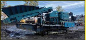
2014 POWER SCREEN 1000 MAXTRAK CONE, 30" DISCH CONV, SCANIA DSL, 16" PADS, 1 OWNER, 3704 HRS \$289,000
