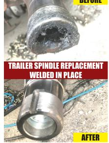
• Drive Spindles From 1 Ton To Class 8 Trucks • Trailer Spindles From 3,500# To Class 8 Axles Spindles can also be repaired by welding up the worn area and then remachining to factory spec. This includes tracing threads or remachining new threads.
