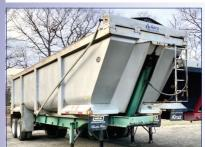
2013 KRUZ 34" x 7' Side Steel Scrap / Demo Trailer: 70,000lb. Center Point Suspension, Electric Ride., Good.Liner,, Electric Tarp, Tarp. Very good condition call for price
