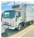
2016 ISUZU NPR-HD Diesel. 142k 16'x91"x96" Insulated Reefer. Carrier 40x. Roll-up Rear Door. Chicago Style Step. Stl#221423, \$42,900
