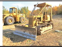
1979 CATERPILLAR D3. 3204, Powershift Transmission, 60% Undercarriage, OROPS With Sweeps, Excellent Condition, Working Daily. $12,500
