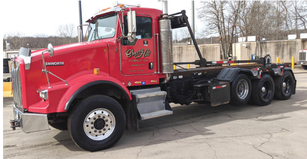
2004 KENWORTH T800 Roll-off , 600,000 miles, 20K Front, 40K Rears, Fixed Pusher Axle, 8 LL Eaton Fuller (1yr old), C15 475 Engine, Galbreath Hoist, Auto Tarp, Auto Can Lockers. Asking $54,000.
