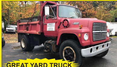
1987 FORD L8000 S/A DUMP. 3208 CAT, 5 + 2 Speed, 10' Body, Asphalt Chute, Body In Excellent Condition, $5,400
