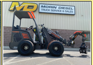
CAST LOADERS. Kubota Diesel, Telescopic Boom, Aux Hydraulics
