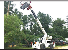
GALION RT-150 ROUGH TERRAIN CRANE. 15 Ton Capacity, 453 Detroit Diesel Engine, 3 Stage Boom, Pin on Manlift Basket, Four Wheel Steer, Four Outriggers, Enclosed Cab. Runs Like New. Steering Cylinders Leak, and Need to be Repacked. $12,500
