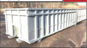
**30-YD HEAVY DUTY** ROLL-OFF, 22' Long, Brand New 1/4" Floor Just Installed, Angled Gussets At Floor And Wall Front To Back, 12" On Center Cross Members, Just Painted, \$4,500.860-205-3190
