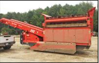
Fn173 2017 TEREX FINLAY 595. 228 Hours, 74 HP, 11x9 Double Deck, Hyd Variable Grid Angle, 6.5 Yd Hopper, 48" Wide Fines Conveyor, Remote Control, \$161,250.
