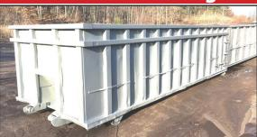
30-YD HEAVY DUTY ROLL-OFF, 22' Long, Brand New 1/4" Floor Just Installed, Angled Gussets At Floor And Wall Front To Back, 12" On Center Cross Members, Just Painted, \$4,500. 860-205-3190
