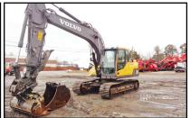
8670 2014 VOLVO EC160DL Excavator, 5K Hours, Coupler, 3rd Valve, Hyd Thumb, 36" Digging Bucket, 63" Hyd Tilt Bucket, A/C/ Heat/ Stereo, 50% U/C, \$108,500.
