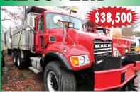
2004 MACK GRANITE 13'6" ALUMINUM DUMP BODY: 3 chutes, 400 MACK, 8LL, 20F/46R, 42.5x22.5 Front 12x22.5 Rear Tires. Set up for Highway Plow. Central Hydraulics. All Sander controls in cab.
