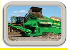
**FOR SALE** \$189,000 5000 Hr Warranty! 2017 McCloskey 512R High Production Trom-mel Screener with Remote Control Grizzly & 16' Radial Stacker, 12' 6" Feed Hopper, 5' x 12' Trommel, 3/4" Screen, Cat C3.4B 120 HP, In Line 4 Cyl. Engine.
