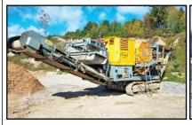
8784 2004 ERIN 1265J 49x26 TRACKED JAW CRUSHER. CAT C9 POWER, 12'-5"X 7'-7" FEED HOPPER, HYD MAGNET, 47" DISCHARGE BELT, 25" SIDE DISCHARGE BELT, \$125,000.
