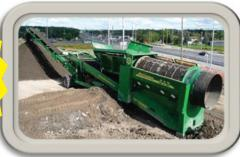
New! 2017 McCloskey 512R High Production Trommel Screener with Remote Control Grizzly & 16' Radial Stacker, 12' 6" Feed Hopper, 5' x 12' Trommel, 3/4" Screen, Cat C3.4B 120 HP, In Line 4 Cyl. Engine.
