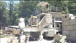
1990 UNIVERSAL 32"X54" PORTABLE JAW CRUSHER. S/N 537X220, 60"x20' Vibrating Grizzly Feeder,
