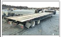
2001 LANDOLL 660 35 Ton Tandem Axle Trailer, Hydraulic Sliding Axle, Air Ride, 10' Upper Deck, 38' Main Deck, 102" Wide, Winch Call For More Information.
