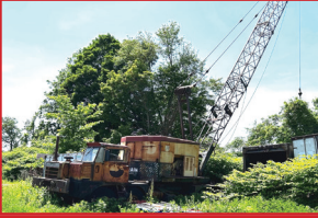
LORAIN CRANE. 40 Ton, Cummins Lower Motor, Detroit Upper Motor, 12' Boom
