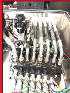
Noreaster Fabrications Custom Central Hydraulic System With Stainless Steel Tank, Enclosure, Integral Filtering, Electronic Ground Speed Control
