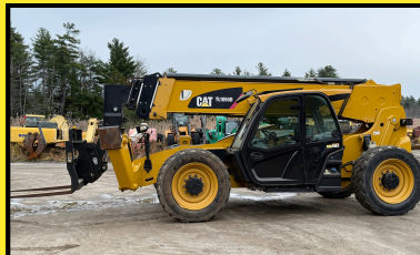
2019 CAT TL1055 10,000LB CPTY, 55' HT, EROPS, A/C, 60" FORKS W/ 72" CARRIAGE, FRONT OUTRIGGERS, 3,287 HRS $99,000
