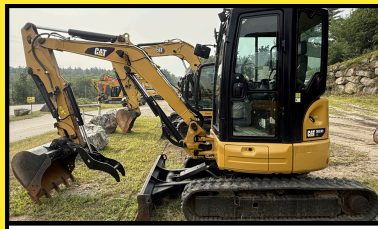
2018 CAT 303.5E2CR A/C, BM SWNG, AUX HYD, 34" BKT, HYD THUMB, BLADE, 16" RBR PADS, 1,580 HRS $45,000
