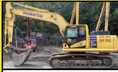
(2) 2022 KOMATSU PC210LC-11 A/C, 9'7" STK, AUX HYD, HYD Q/C, 42" BKT, HYD THUMB, TIER-4 FINAL DSL, PTRN CHNGR, 32" TG PADS, 1,680+ HRS $209,000 EACH
