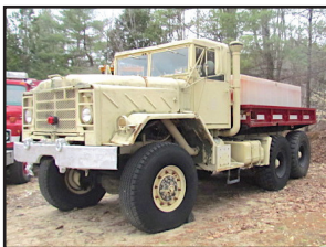
6x6 Auto Brush Poly Tank & Pump Unit.
